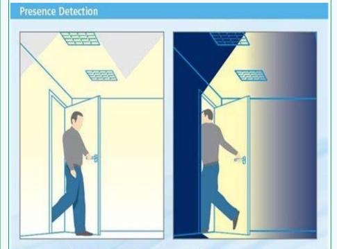
Detectors will switch on lighting automatically when a person enters the room, and switches off lighting automatically when no movement is detected.
